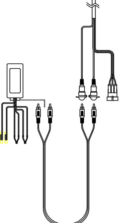
Connect the SNI35 to the JMP5W800 using an RCA audio cable.
